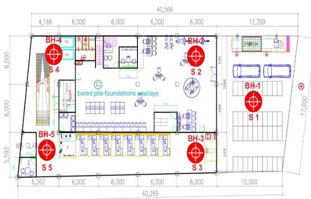
Figure 1. Drill points and boredpile locations analyzed
