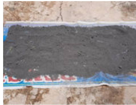
Figure 2. Drying process of the Palm Shell Ash
