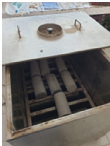
Figure 1. Steam curing machine
