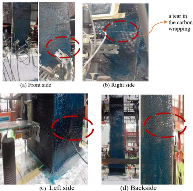
Figure 17. Damage pattern in the second step
